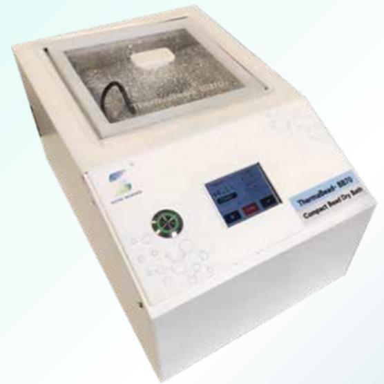
**Interface :** Features a 2.3-inch touch display with an intuitive interface for monitoring and control, along with support for program customization and memory storage.
